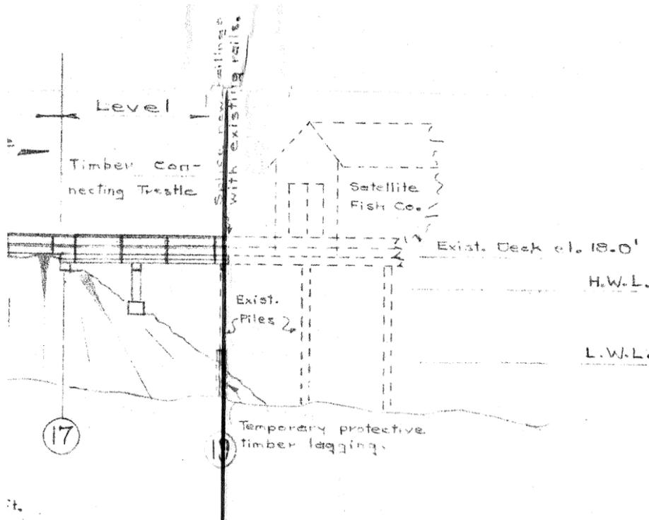
Figure 1 – Top of Wharf Elevation in Chart Datum (Ref 1)
