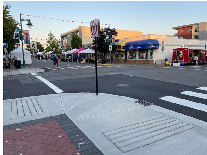
Crosswalk at Beacon Avenue and 4<sup>th</sup> Street in Sidney, BC. Multiple residents and staff commented on the improved safety and accessibility of this intersection with the addition of reduced corner radii and tactile walking surface indicators. Photo Credit: Kaila Hunte, Left Turn Right Turn
